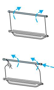
7. Insert the shade into the side mounting brackets and check to make sure that it operates properly.
